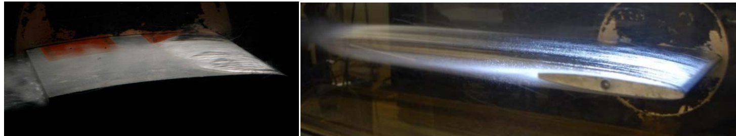
Partial sheet cavitation (above) and supercavitation (below) on a NACA0009 profile.
